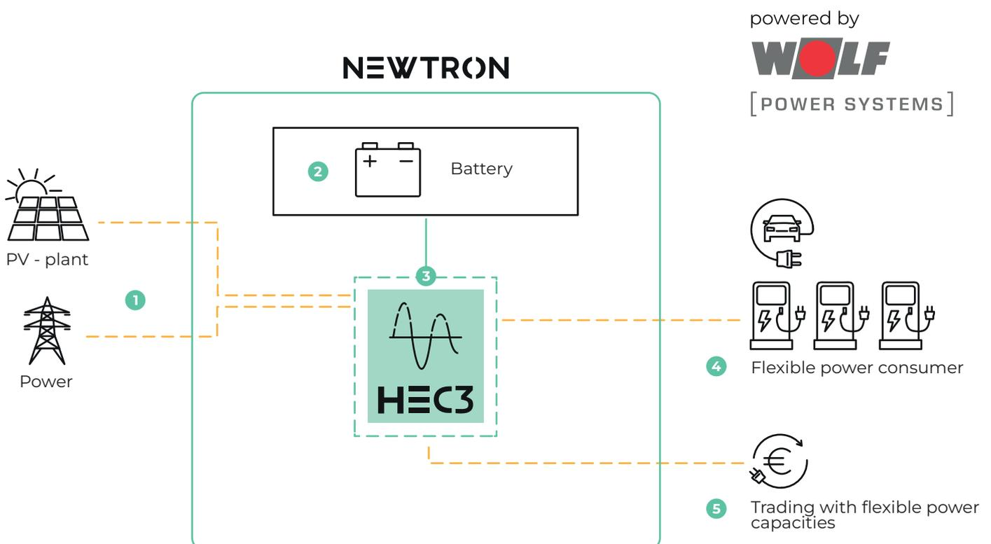
The HEC3 management is the core and the standardized interface to the energy components, which are identified and controlled according to demand. With the energy management system HEC3, energy flows are identified and flexibilities are actively traded on the electricity market.
