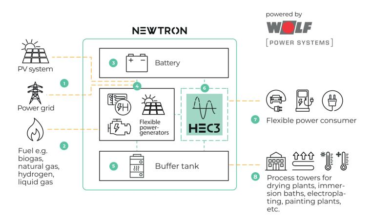
HEC3 is the managing core and possess the standardized interface to different energy components, which are configured as requested. With the HEC3 energy management system, energy flows are identified and flexibilities are actively traded on the electricity market.
