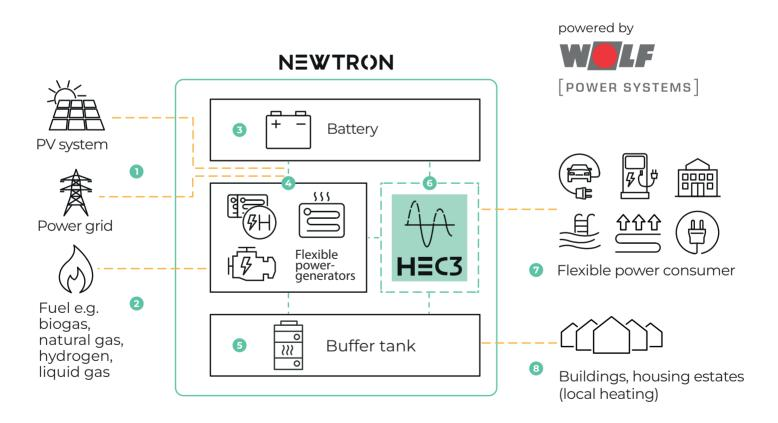
HEC3 is the managing core and possess the standardized interface to different energy components, which are configured as requested. With the HEC3 energy management system, energy flows are identified and flexibilities are actively traded on the electricity market.
